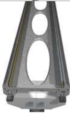
75-foot Guideway Section
